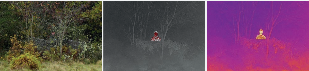
TIR LC TARP. OBJECTS: Person in BDU standing behind TIR LC Tarp.
