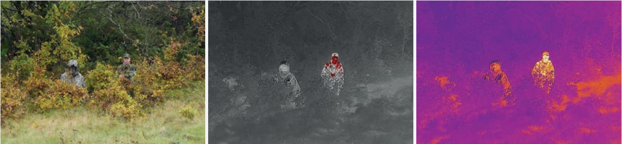
TIR LC PONCHO. OBJECTS: Person 1 in BDU, combat vest, helmet, and TIR LC Poncho. Person 2 in BDU.
