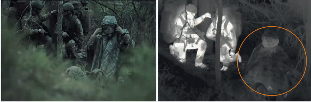
TIR LC PONCHO. Person 1 and 2 in BDU. Person 3 in BDU, combat vest and helmet, covered with a TIR LC Poncho.
